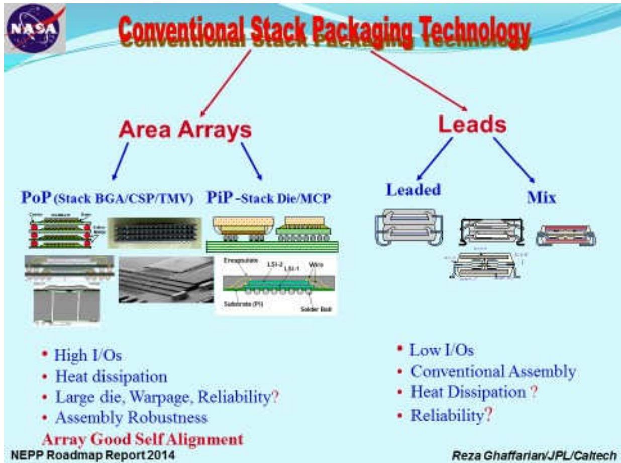
Figure 4-2. 2.5/3D packaging technologies showing conventional to advanced configurations.
