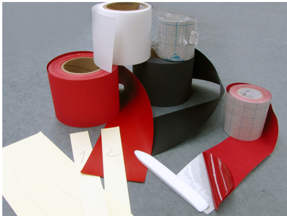
Filmoplast T (at right) and Archival Products' C-cloth slit to custom widths. 10pt folder stock for spine-stiffeners.
