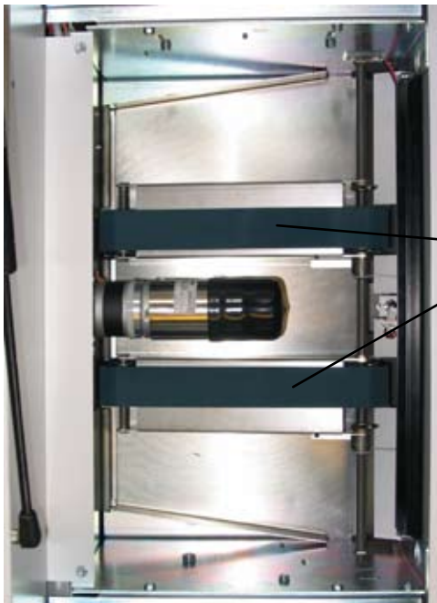
Upper feed belts in normal position.
