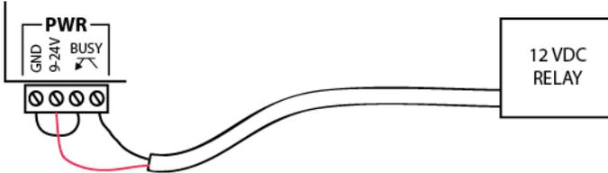
In the example above the BooTunes is being powered by a 12 VDC power supply using the barrel connector in the back. The busy output is borrowing power from this power supply to power the relay. The load voltage must match the BooTunes power supply voltage when connected in this way.
