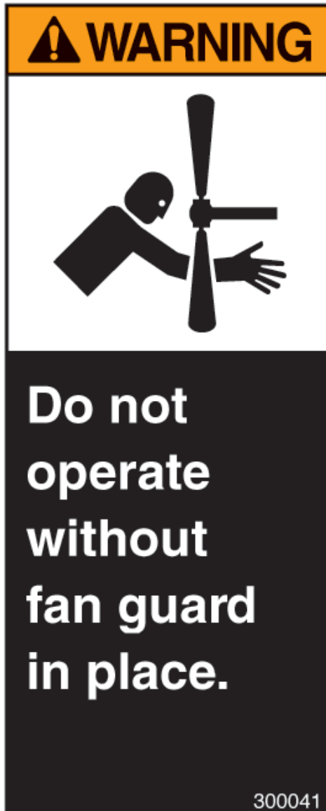
Figure 5. To be placed near oil cooling fan. P/N: 300041
