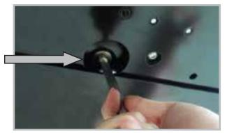
Undo the bolt and let the oil drain into an open top container which can hold a minimum of 2 litres.
