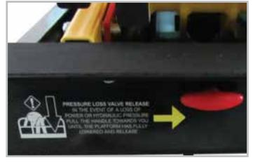
Emergency pressure loss valve release handle
