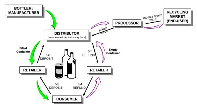
With this system, the distributors address the transporting and processing systems/facilities to handle the returned containers. The processing facilities handle aluminum, PET (polyethelene terephthalate), and glass containers. The retailers address the counting and sorting of returned containers by distributor groups and the storing of the containers.
