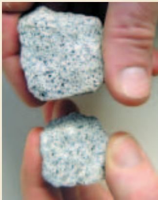
Don Borkowski holds two samples of granite, the top from the "new" supply of replacement stones, and the bottom from the chapel towers, showing that they are an exact match.
