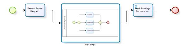
**Diagram 14.** Expanded Sub-process Example
