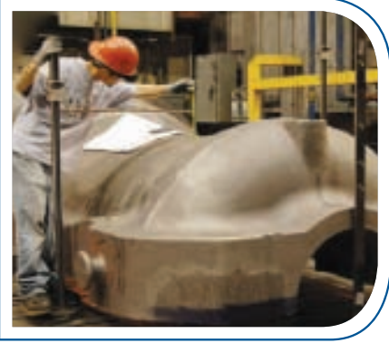
Large steel turbine housing
