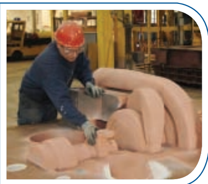
Molding/core making (complex pump housing)
