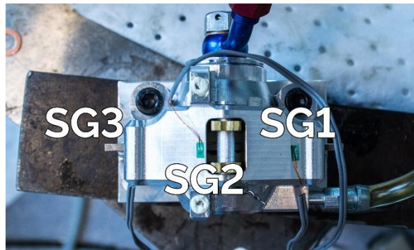
Figure 14: Strain gauges mounted on rear caliper.
