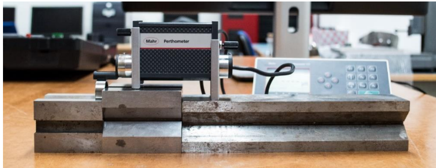
Figure 11: Perthometer setup. Investigated specimen in the left field of the picture.
