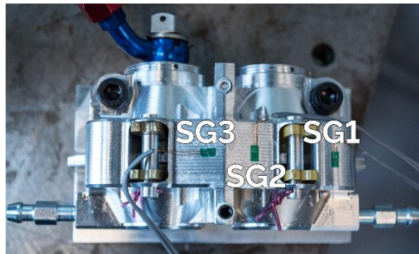
Figure 13: Strain gauges mounted on front caliper.
