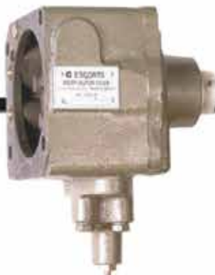
Pressure transformer DU Same effect as KR1, but with additional two-stage variable load braking. ( basic valve with DU = Distributor type KE 2 - A, B or C, depending on the type of 'empty-loaded' change-over device )
