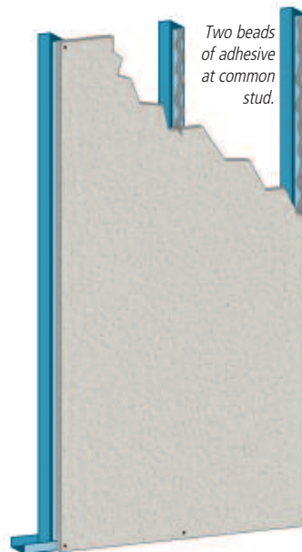
Nailing or screwing is required only at top and bottom of prefinished gypsum panels when adhesive is applied and panels are prebowed to give pressure at the center of the board.
