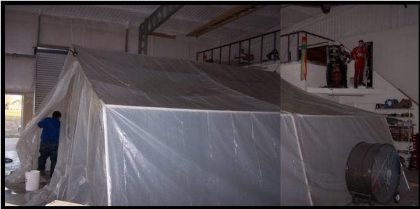
PVC and plastic make up the outer shell. Jason wanted to be able to put the whole aircraft in the booth, so it got BIG.
