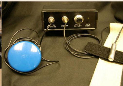
The vibrotactile device shown above was used in previous NIH studies. A more clinical form that is easy to use is being developed. Dr. Christy Ludlow (r) created the vibrotactile device.
