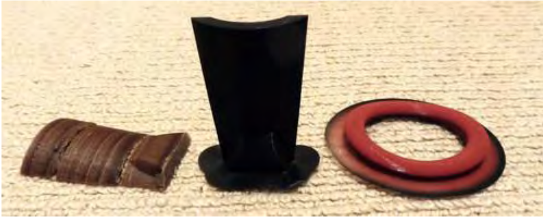
Prototypes 44, 45, and 46 as they printed, with brims at the bottom for stability, before trimming.
