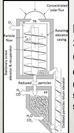
Latest Sandia Reactor Concept for beam down power tower (moving packed bed, spatial pressure separation)
