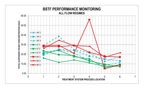
There is little if any demonstrated benefit in solids settling in the first solids settling basin (Location 2). Some limited solids settling effectiveness is demonstrated in the aerobic zone.
