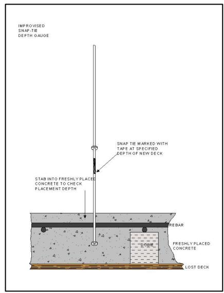
Figure 2.2-1. Diagram of How to Use an Improvised Snap Tie Depth Gauge.
