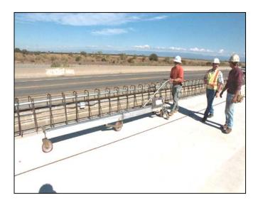
Figure 6.1-1. Smoothness Testing, per California Test 547.
