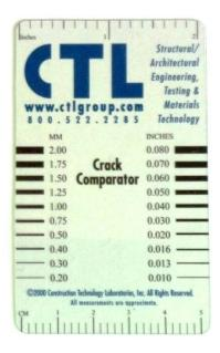
Figure 6.1-3. Crack Comparator Makes Checking Crack Width Easier.
