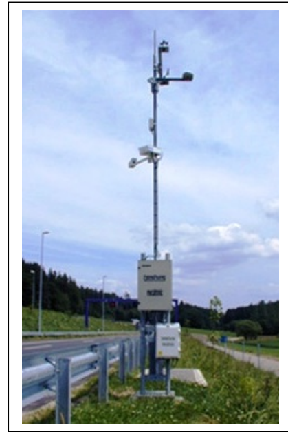
Typical NHDOT Non-Invasive Pavement Sensor System
