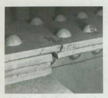
Fig. 67. Fatigue crack in cantilever bracket connection plate
