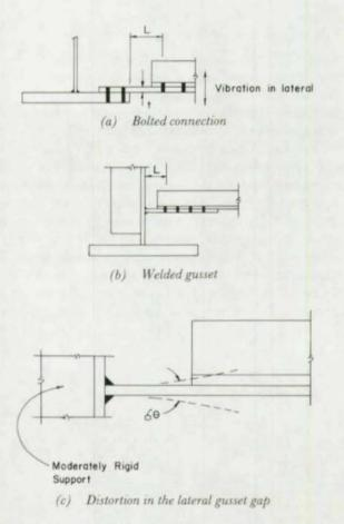
Fig. 64. Schematic of vibration displacement at lateral gussets
