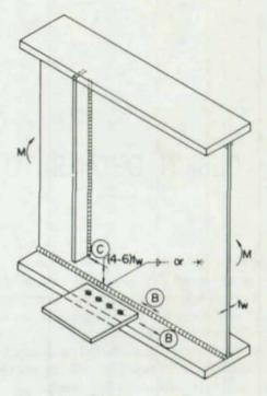
Fig. 3. Bolted flange attachment
