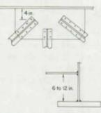
Fig. 63. Suggested lateral gusset plate at points with no transverse stiffener
