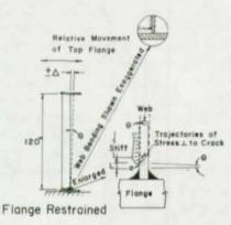
Fig. 50. Schematic showing deformation of web between end of stiffener and flange when lateral sway occurs
