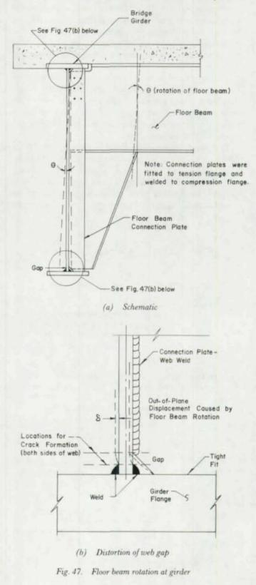
moment regions that are not near the end reactions do not develop as much out-of-plane flexing of the web, or a relative displacement in the gap region, due to the ability of the entire girder to accommodate this rotation by deforming with the floor beam. Whether or not this region can become a problem depends on the lateral stiffness of the girder flange.
