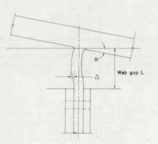
Fig. 42. Schematic of out-of-plane deformation in gap length
