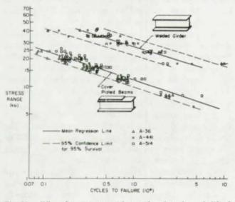
Fig. 28. Effect of stress range and type of steel on the cycle life of coverplated and plain welded beams
