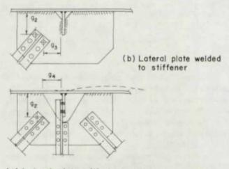
(c) Lateral plate with transverse member bolted to stiffener
