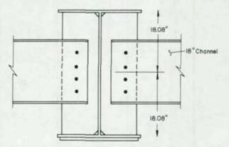
Fig. 17. Stiffener plates for diaphragm connections
