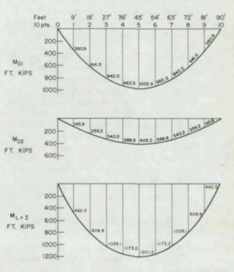
Fig. 15. Moment diagrams (truck loading)
