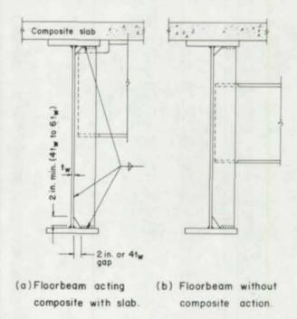
Fig. 51. Recommended floor beam connection plates for negative moment regions and near end supports
