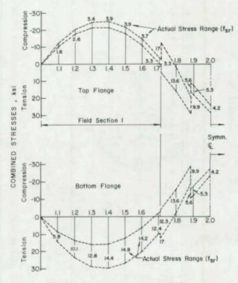
Fig. 20. Combined stress diagrams (S/5.5)
