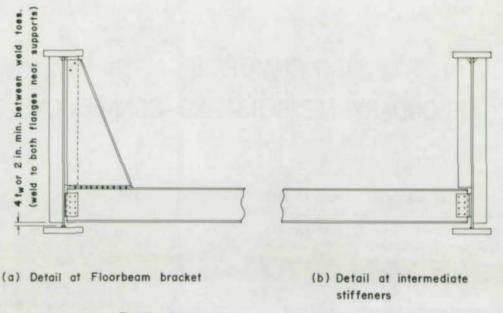
Fig. 52. Suggested floor-beam-to-girder connections
