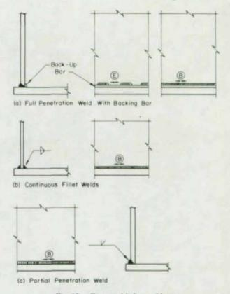
Fig. 12. Cover welds for steel boxes
