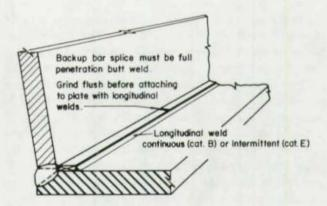
Fig. 77. Schematic showing butt splice in backing bar
