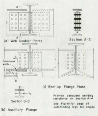
Fig. 39. Recommended connections where stringer flanges must clear floor beams (see Fig. 45a for stringer connection)
