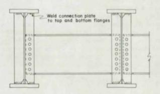
Fig. 70. Diaphragms and connection plates for skewed bridges
