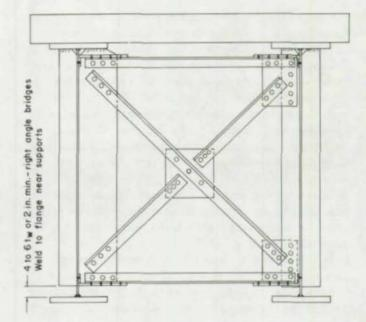
Fig. 56. Cross-frame details with improved fatigue strength for straight right-angle bridges
