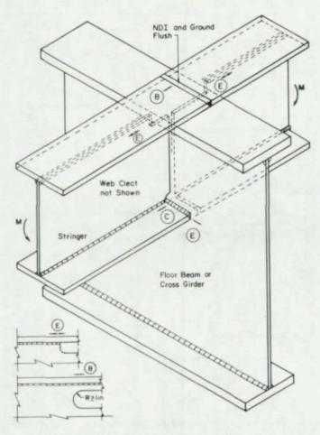
Fig. 13. Floor beam-to-girder connection with continuous floor beam flange
