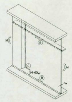
Fig. 7. Transverse and longitudinal stiffeners placed on opposite sides of web
