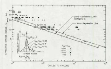
Fig. 32. Comparison of variable load tests with mean and lower confidence limit for Category E using RMS effective stress range (Ref. 21)
