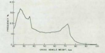
Fig. 25. Gross vehicle weight distribution from 1970 FHWA Nationwide Loadometer Survey
