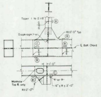
NDI groove welds when stresses are perpendicular to weld
