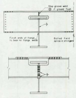
Fig. 14. Stringer-to-floor beam connections with high allowable fatigue strength
