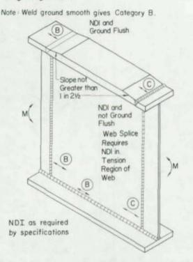
Fig. 8. Transverse groove welds in web and flange
