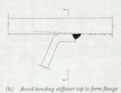
Fig. 73. Attaching stiffeners to deck plate
