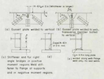
Artach stiffener to flange in curved girder bridges and where aut-of-plane movement may be large.
