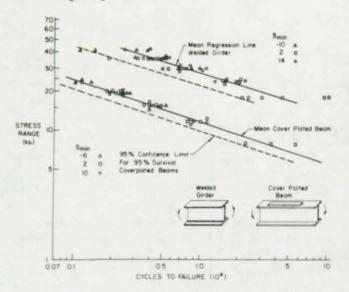
Fig. 27. Effect of minimum stress and stress range on the cycle life for the welded end of coverplated beams and plain welded beams
