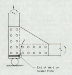
Fig. 69. Schematic of crack in gusset plate of truss caused by secondary stress
