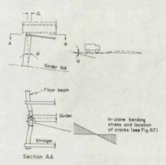
Fig. 66. Schematic of deformation introduced into floor beamcantilever bracket splice plate (see Fig. 65)
