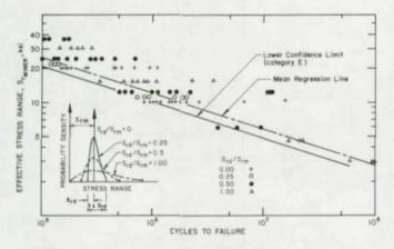
Fig. 31. Comparison of variable load tests with mean and lower confidence limit for Category E using Miner's Rule (Ref. 21)
