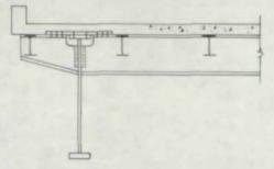
(b) Girder bridge with stringers framing into floor beam and connection plate embedded in slab
