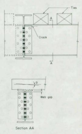
Fig. 41. Schematic of web cracking from flange rotation
