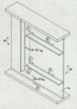
Fig. 6. Transverse and longitudinal stiffeners
