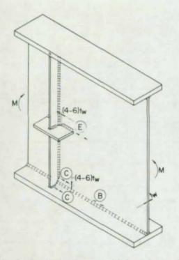
Fig. 5. Bracket attached to beam web in lower stress region
