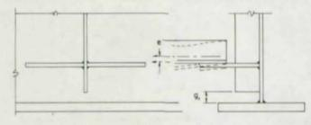
(a) Lateral connection plate at vertical stiffener
