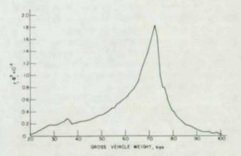
Fig. 26. Probable damage caused by various truck weights
