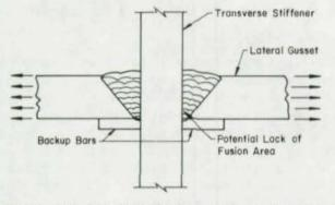
Fig. 76. Schematic of lack-of-fusion area when backup bar is perpendicular to stress field
