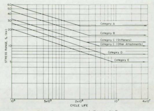
Fig. 30. Design stress range curves for Categories A to E
