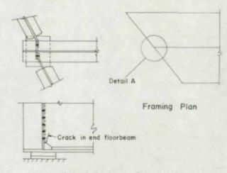
(a) Detail A as built, showing fatigue crack location
