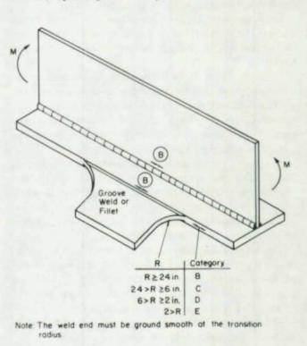
Fig. 4. Radiused transition for welded flange attachments
