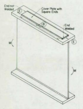
Fig. 10. Coverplated beam showing region of critical fatigue stress
