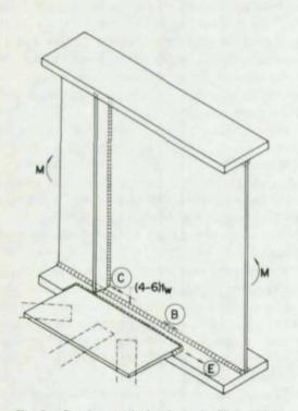
Fig. 2. Bracket attached to flange by fillet welds
