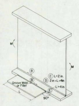
Fig. 1. Bracket attached to flange by longitudinal fillet or groove welds
