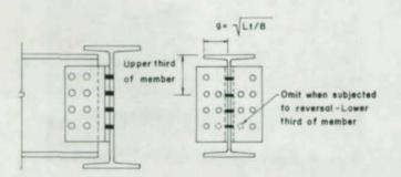
Fig. 40. Recommended configuration of outstanding legs of simple end connections (also see Fig. 45a)
