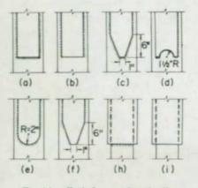
Fig. 11. End of cover plate details
