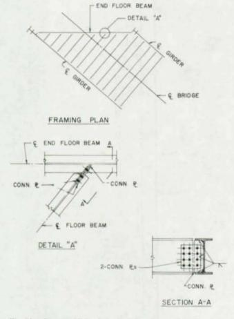
Fig. 72. Suggested "simple" connection at skewed end floor beam
