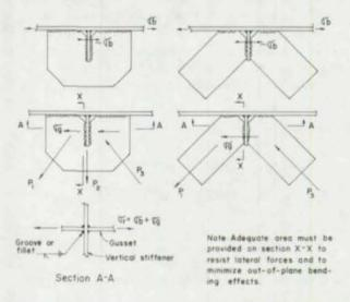
(a) Diagrammatic only-usual gusset (b) Lateral gusset with substantial provides much greater reduction in cross-sectional area cross-sectional area on X-X.
