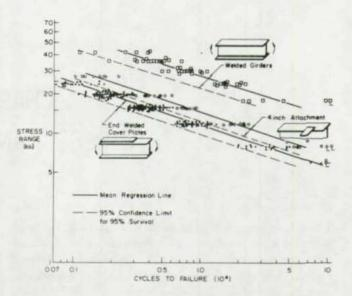
Fig. 29. Comparison of short welded attachments with coverplated and plain welded beams
