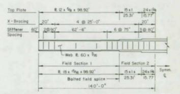
Fig. 19. Girder section required by load factor design—dead and non-cyclical live load
