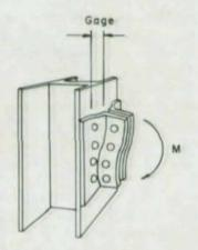
Fig. 33. Deformation of standard beam connection
