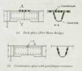
Fig. 75. Deck panel splices
