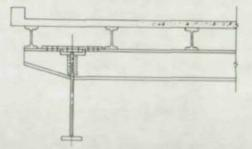
(a) Girder bridge with stringers on top of floor beam
