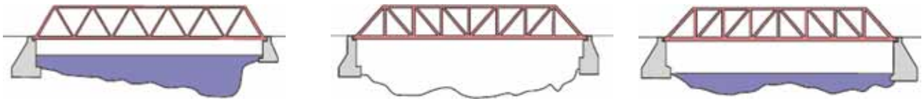
(a) (b) (c) Figure 4 Three types of truss bridge design: (a) Warren Truss, (b) Pratt Truss and (c) Howe Truss ( http://www.matsuo-bridge.co.jp/english/bridges/basics/truss.shtml )
