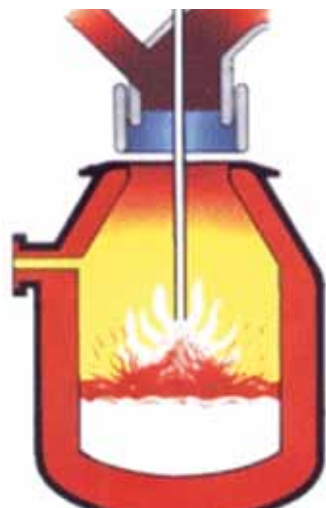
Figure 3 – Schematic diagram of a BOS vessel showing the lance blowing oxygen through the liquid iron. ( http://www.coruselearn.com/images/bos.gif )
