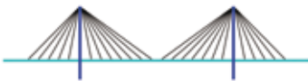
Figure 1a Fan design of cable-stayed bridge in which the supporting cables all originate from the top of the tower. ( http://en.wikipedia.org/wiki/File:Bridge-fan-cable-stayed.svg )
