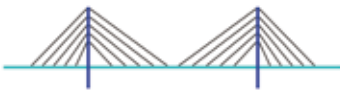
Figure 1b Harp design of cable-stayed bridge in which the supporting cables are situated down the length of the tower. ( http://en.wikipedia.org/wiki/File:Bridge-harp-cable-stayed.svg )
