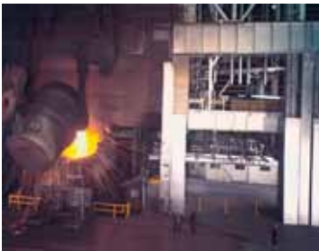
Figure 2 – Charging a BOS furnace. An idea of the scale of the furnace is given by the size of the two people. ( http://www.wrhs.org/index.php/crawford/Online_Exhibit/Clev_Steel/Part3 )
