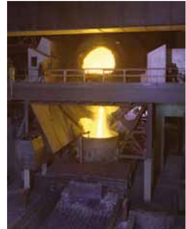
Figure 4 – Tapping a BOS furnace. ( http://www.wrhs.org/images/uploaded_images/caam/Cleveland%20Steel/Making%20Steel/WarrenBOFTapping.jpg )
