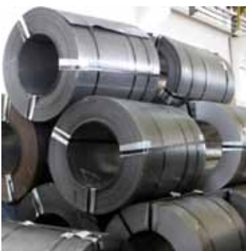
Figure 9 – Rolls of cold rolled strip steel. ( http://www.nskamericas.com/cps/nsk/eu_en/p/images/content/CS_7003_ImageR_square_rdx_95.jpg )
