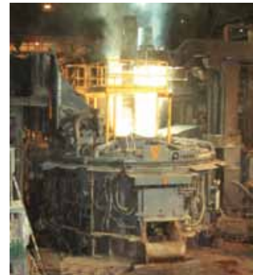
Figure 5 – Electric arc furnace for secondary steelmaking. ( www.scienceinpublic.com )
