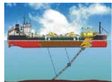
Figure 8 - Diagram showing trailer dredging process for extraction of marine sand and gravel.
