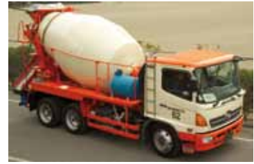
Figure 3 – Mobile cement mixer used to keep concrete moving until it is poured. ( http://upload.wikimedia.org/wikipedia/commons/2/20/CementMixerM2439.jpg )
