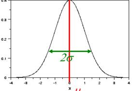
• The variance is related to the 2<sup>nd</sup> order non-central moment by  $\sigma^2 = E[(x - \mu)^2] = E[x^2 - 2x\mu + \mu^2]$  $= E[x^2] - 2E[x]\mu + \mu^2 = E[x^2] - \mu^2$
