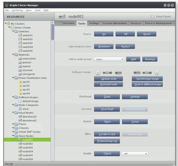
By selecting a cluster node in the tree on the left and the Tasks tab on the right, you can execute a number of powerful tasks on that node with just a single mouse click.
