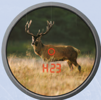
After the distance is displayed, H 23 appears. The hunter must aim 23 cm over the aiming point on the target.
