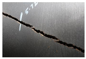
The opening of the crack and lateral displacement indicated high residual stress that remained in the material from the casting process. Applied stresses are those that are caused by external loading on the component as part of its use or operation in service.
