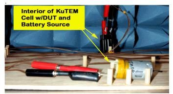
Figure 4. Baseline DUT shown inside KuTEM Omni-Cell
