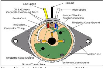
Figure 13. Typical X2Y placement inside a DC Motor
