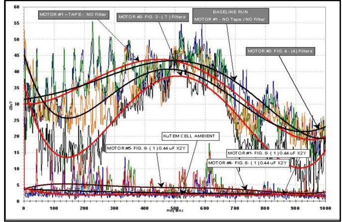
show that use of the tin-plated copper foil tape had minimal effect on the RF noise suppression of the motors and has been disregarded by the authors as a significant factor in achieving the results obtained.
