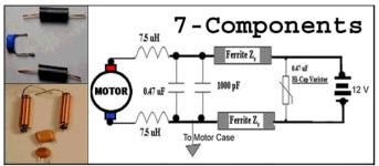
Figure 6. (7) Component Motor Filter Network.
