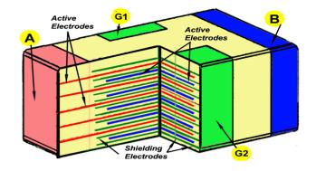
**Figure 9.** *X2Y<sup>®</sup> Shielding Electrode Architecture*
