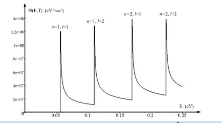
Figure 1. Dependence of density of states of 1D electron gas of energy  $L_1 = 10^{-8}$  and  $L_2 = 1.5 \times 10^{-8}$ .
