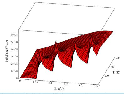
Figure 3. Dependence of density of states of 1D electron gas on the energy and temperature in threedimensional space:  $L_1 = 10^{-8}$  m and  $L_2 = 1.5 \cdot 10^{-8}$  m.
