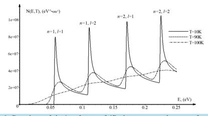
Figure 2. Dependence of density of states of 1D electron gas on the energy for different temperatures:  $L_1 = 10^{-8}$  m and  $L_2 = 1.5 \cdot 10^{-8}$  m.
