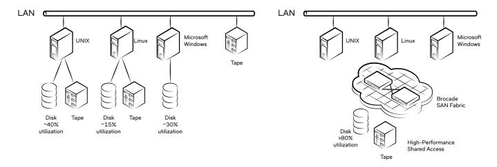
Figure 1: A Brocade SAN-based consolidation solution can significantly improve data availability and resource utilization.
