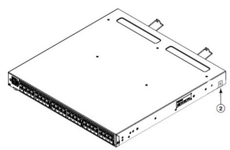
Figure 19 - Brocade 6510 right side seal application
