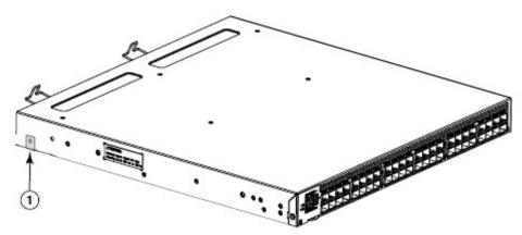
Figure 18 - Brocade 6510 left side seal application
