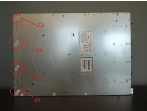
Figure 24 - Brocade 6520 bottom side seal locations
