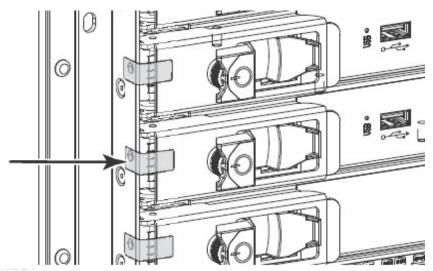
Figure 14 - Brocade DCX-4S and DCX 8510-4 Backbone flat ejector handle seal application
