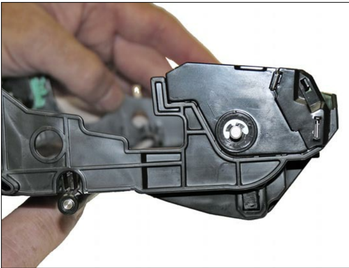
16. Install the E-ring on non-gear side of the drum axle shaft. Press the axle bushing in slightly so that the e-ring slot is accessible.
