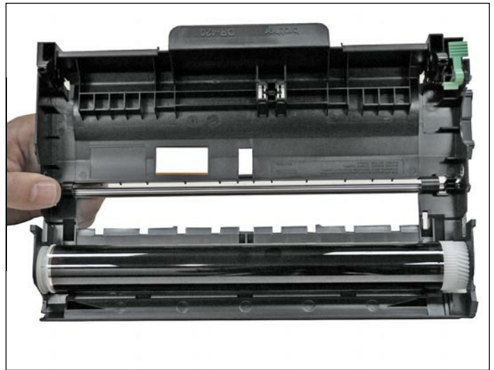
11. Install the drum, hub side first. You will have to compress the hub spring slightly for the drum to fit properly.
