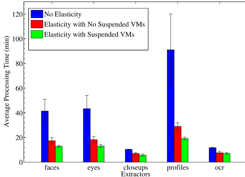
Processing time is reduced by 70% and 80% if started with suspended VMs
