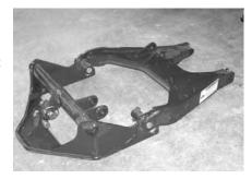
3. Raise the attachment arm and position it to the vehicle mounting frame. Install the two pins and retainer pins.
