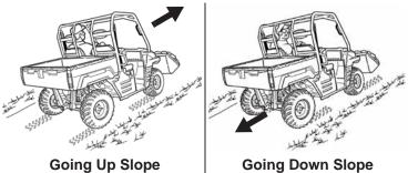
With a loaded bucket and an empty cargo box, go up or down the slope with the heavy end toward the top of the slope. Look in the direction of travel.
