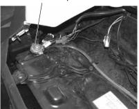
5. Reinstall the pressure cap. Use of a non-standard pressure cap will not allow the recovery system to function properly. Your POLARIS dealer can provide the correct replacement part.
