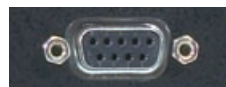
The SP 2’s RS 232 port allows for the integration of external control systems (AMX, Crestron, etc).
