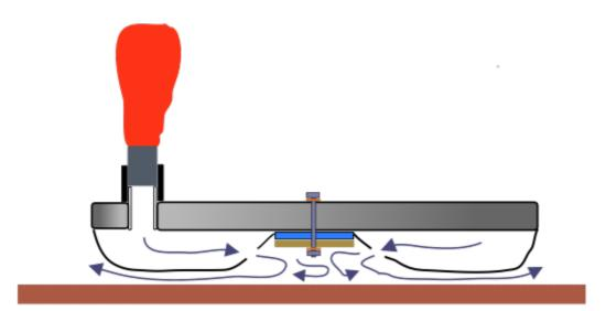
holes from the floor and forms an 'air barrier' to the escaping air. The air trapped in the inner 'donut-hole' slowly leaks between the 'skirt' and floor and forms an "air cushion" that provides a constant padding of air.
