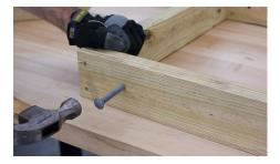
Connect part (C) to part (A) with a \[ 3\% \] carriage bolt. Use a hammer if needed.
