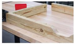
Tip: When arranging the rectangle frames for both sets, put the two (A)s with the handle cutout in a mirroring orientation so that, when fully assembled, the plywood board will be on the inside of the person carrying the set.
