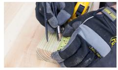
At the top of part (C), mark a point that is 1 34" from the top and 1 34" from the edges. This is the center of the circle.
