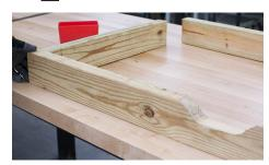
**Tip:** Direct-measure your board stock's width and use half of this number in place of the 1 ¾" for a more precise mid-point. 1 ¾" is based on a 3 ½"-width 2x4.
