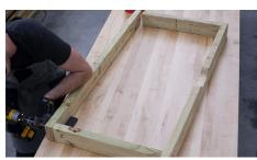
Use two 2 1/2" wood screws at each corner to attach the boards to each other.
