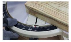
At the bottom of part (C), mark a line at a 29° angle from one of the corners. You can also use a compound miter saw to dial in to 29° if you have one.
