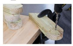
Using a \%" drill bit, make a hole at the center of the circle you marked.
