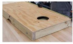
Attach at the four corners using 1 1/2" wood screws. Then use screws at 12-inch intervals along the perimeter of the board.
