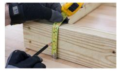
On the outside of part (A), mark a point 4" from the left edge and 1 34" from the top edge.
