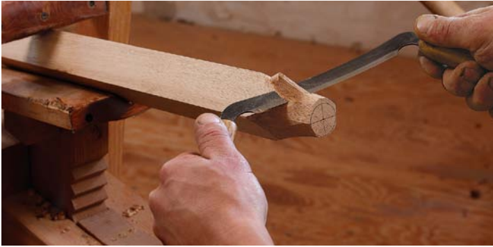
Narrow the end first. Fischer uses a drill-mounted cutter (below) to make the tenons. Before using the tool, you need to narrow the end using a spokeshave or drawknife (above). Draw a circle on the end as a guide.
