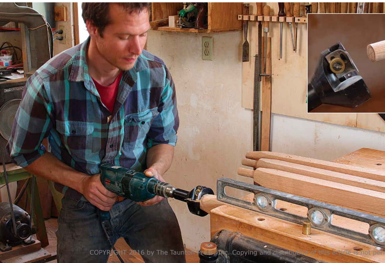
Pop in a stop. The cutter makes 3-in.-long tenons—too long for this stool—so Fischer inserts a dowel into the cutter to act as a stop.
