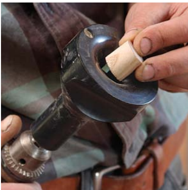
Pop in a stop. The cutter makes 3-in.-long tenons—too long for this stool—so Fischer inserts a dowel into the cutter to act as a stop.
