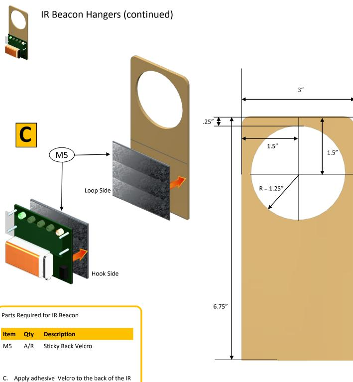
C. Apply adhesive Velcro to the back of the IR Master Beacon, and to the IR Beacon Hanger between the pencil marks. Place the loop side of the Velcro onto the hanger, and the hook side on to the IR Beacon. Important: Be sure to cover the entire back surface of the IR Beacon with Velcro.
