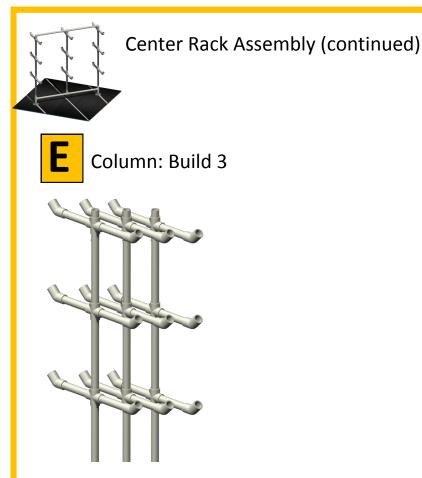
Note: Lay the pieces flat while assembling to ensure all the angles are straight. Ensure all pipes are seated fully into the fittings and Pegs on all columns align properly as illustrated.
