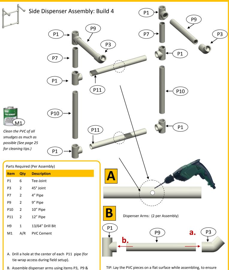
P1. Apply PVC cement to the insides of the joints. Assemble in the recommended order shown. (a, b, c. . .)
