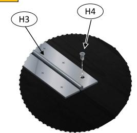
Position the pin portion of the hinge so that it is away from the boards and there is no gap between the boards.
