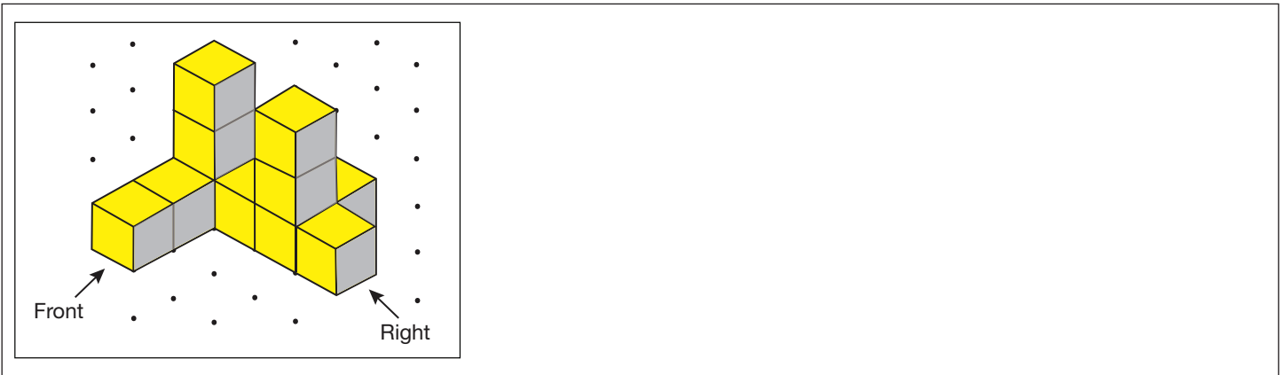
Figure 11. This shows an isometric drawing; draw the orthographic views of the front, right, and top.
