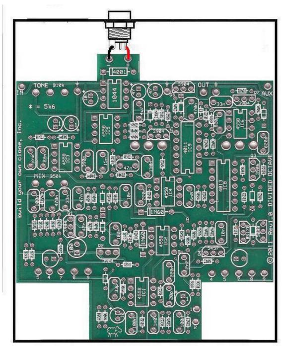
**Step 2:** Connect the TIP (negative) terminal of the DC adapter jack to the "-" eyelet on the PCB with 2 inches of hook up wire. Connect the SLEEVE of the DC adaptor jack to the "+" eyelet on the far right side of the PCB with 2 inches of hook up wire. Connect the battery disconnect terminal of the DC adaptor jack to the "+" eyelet more towards the center of the PCB with 2" of hookup wire. Load the wires in from the bottom of the PCB and solder on the topside.
