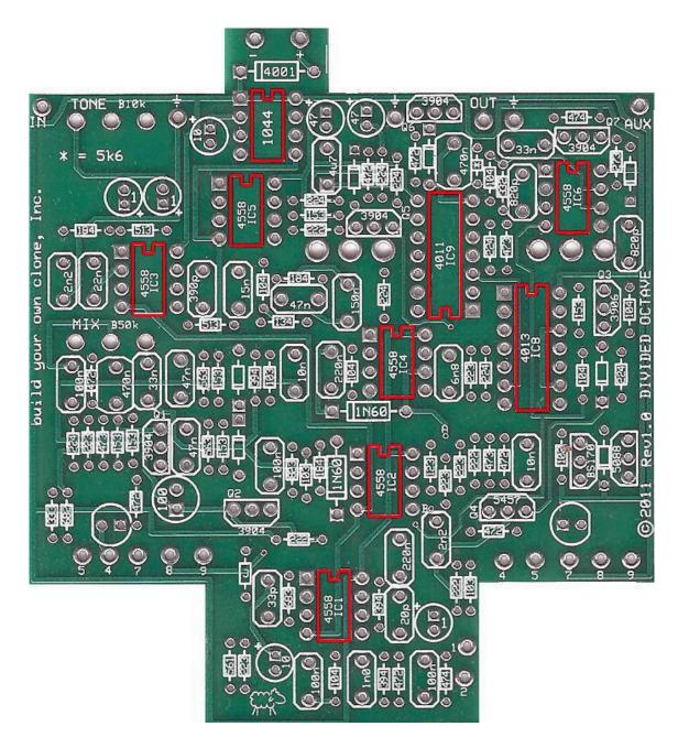
Step 3: Add the IC sockets. Just the sockets!!!! Do not add or solder the actual ICs themselves yet. The ICs never get soldered. Only the sockets get soldered. You will install the actual ICs at the very end of this build.
