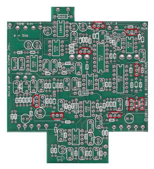
Step 5: Add the Transistors. Orient the transistors so that the flat side of the tansistor body matches up with the flat side on the PCB layout. There are 5 different transistors in this build and it is very important that they each go in their correct place. Be sure to take the time to differentiate the different transistors.
