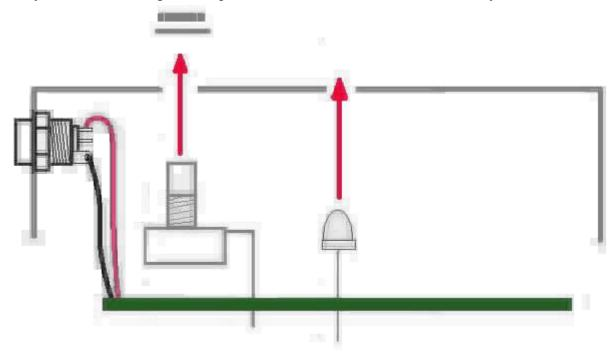
pots and LED all go into their respective holes. Once the PCB assembly is in place, secure it by screwing on the washers and nuts for the pots and toggle switch. Only tighten them with your fingers. You do not want them very tight yet. Be sure to keep your hand on the PCB so that it does not fall off the PC mounting posts of the pots and toggle switch.
