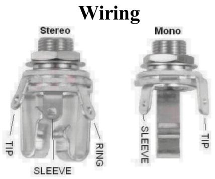
Step 1: Install the 1/4" jacks to the enclosure. The Divided Octave only uses mono jacks. Be sure to install the jacks so that the prong of the IN JACK is at 12 o'clock and the prongs of the OUT and AUX JACKS are are both at 4 o'clock.
