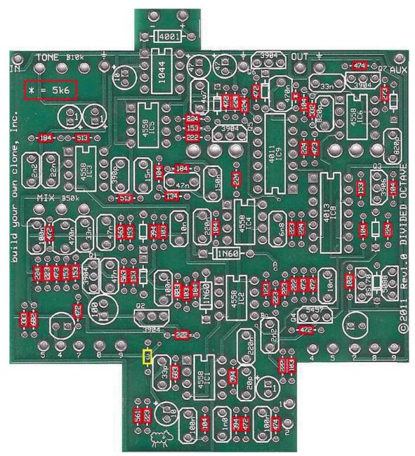
STEP 1: Add the resistors . Resistors are not polarized, so it does not matter which end goes in which solder pad. Take your time and be sure not to confuse similarly banded resistors such as the 470k with the 4k7 or the 22k with the 2k2. If you have difficulty reading the color bands, use a digital multimeter to test the value of each resistor. Note1: The resistor space marked with "\*" is a 5.6k.
