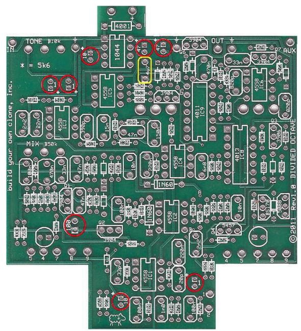
STEP 6: Add the aluminum electrolytic capacitors. These are polarized. The positive end will have a longer lead and should go in the square solder pad. The negative end will have a shorter lead with a black or white stripe running down the body of the capacitor.
