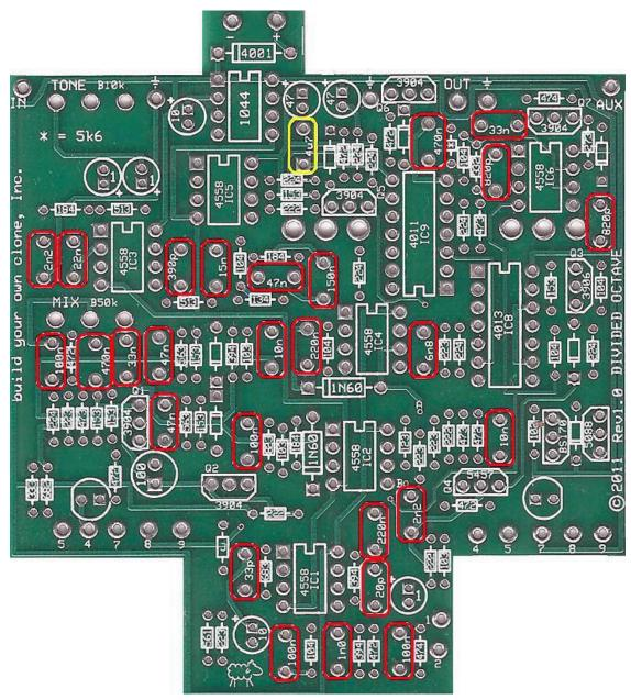
Step 4: Add the film capacitor. These are not polarized and can be inserted into the PCB either way.
