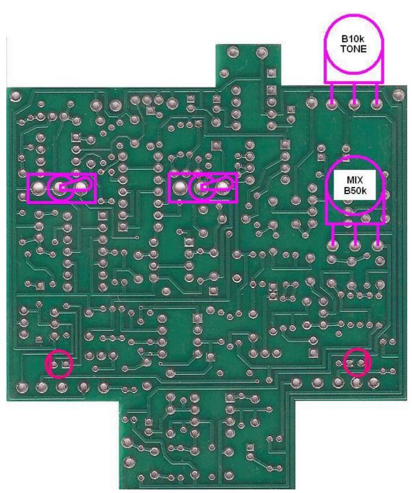
Step 3: Flip the PCB over so that the bottom or solder side is up. Insert the B10k(TONE), B50k(MIX) potentiometers, the two SPDT Toggle Switches, and the two LEDs into the bottom side of the PCB. DO NOT SOLDER ANYTHING YET!!!
