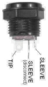
Step 1: Mount the DC adapter jack to the enclosure.
