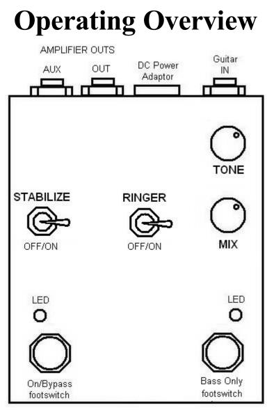
**MIX:** Blends the Octave down and Ringer with clean signal. Full-turn clockwise is pure clean signal. Full-turn counter-clockwise is pure octave signal.
