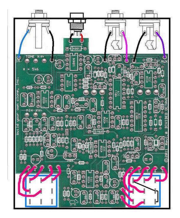
Step 3: Connect the pre stripped and tinned wires to the 1/4" jacks. Step 4: Cut, strip, and tin the footswitch wires.
