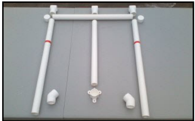
Mounting legs identified by red electric tape
