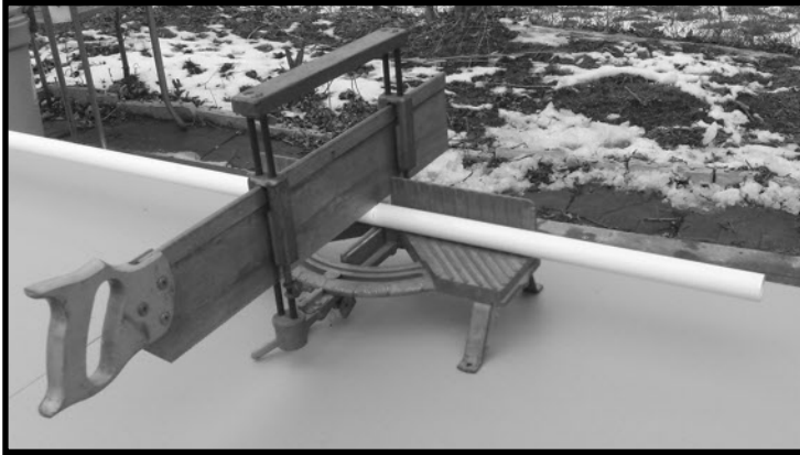
Miter saw steadies work piece for cutting
