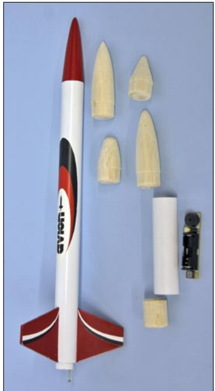
Figure 1: The Avion rocket can easily be upgraded to carry an altimeter payload and be used as a science fair rocket to study aerodynamics. A popular experiment is to see which nose cone shape is most efficient.
