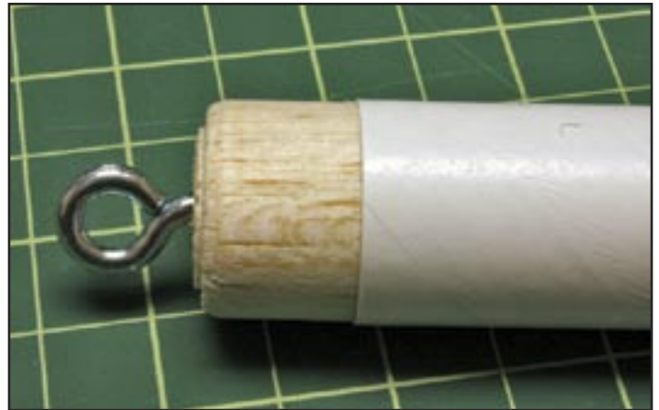
Figure 7: The coupler inserted into the bottom end of the payload bay tube.
