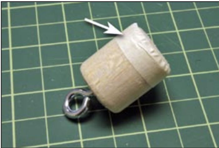
Figure 6: To adjust the fit of the coupler, wrap tape around the forward end to achieve a tight fit.
