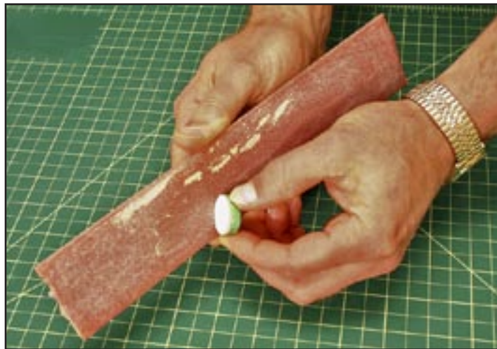
Figure 5: Sand off any overlap that prevents the disk from fitting into the payload bay tube.
