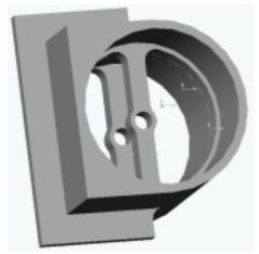
Figure 8: Solid Works Drawing of Thruster Housing
