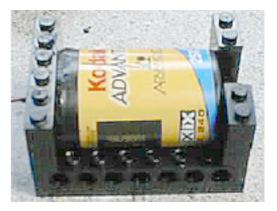
Figure 3: Waterproof Motor Setup
