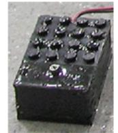
Figure 12: Sealed, Finished Pressure Sensor
