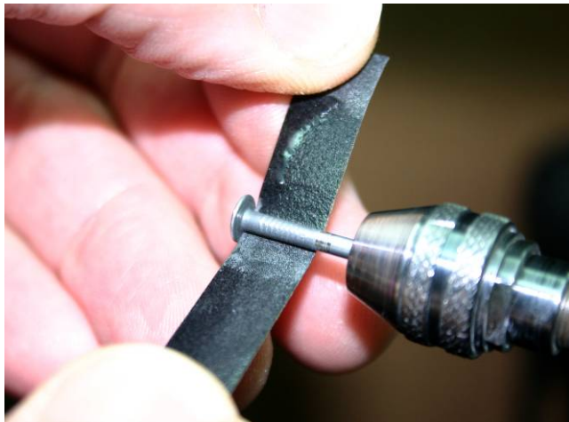
Wet sanding axle shaft
