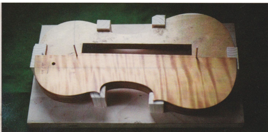
Template in position prior to marking out.
