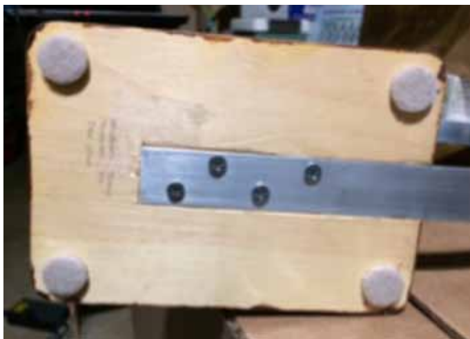
The wooden plaque base is slotted to receive the stand arm made from a 24" aluminum bar.
