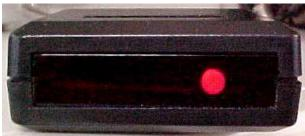
Transmit LED displays easily through the RED lens face.
