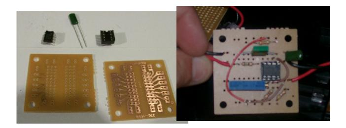
I also learned that it would be better to attach the LEDs remotely, instead of on the board with the other components of the circuit. Lastly do yourself a favor and use board-mounted sockets for your ICs. The heat from the soldering iron could damage the chip.
