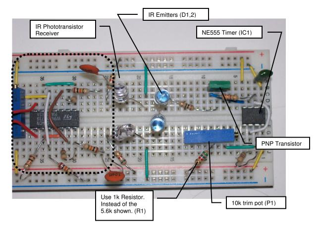
Above is a picture of the breadboard that I created. I was able to get this working fairly easily in the mockup. I initially used LEDs to see if the circuit was working. Then I found out that the CCD in electronic cameras is sensitive to the wavelength of the IR emitter. Use real-time viewing to see the bluish glow emitted from the IR sensor. What we see in the picture is the reflection of the camera flash.
