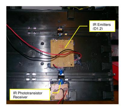
Below you can see the remotely mounted emitter diodes. I use circuit boards to mount the LEDs, It creates a means for mounting and securing the diodes to the track without damaging the diodes themselves.
