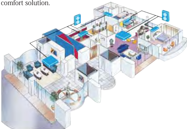
Fig. 3-6-1A PUMY-P-NHMU piping scheme
