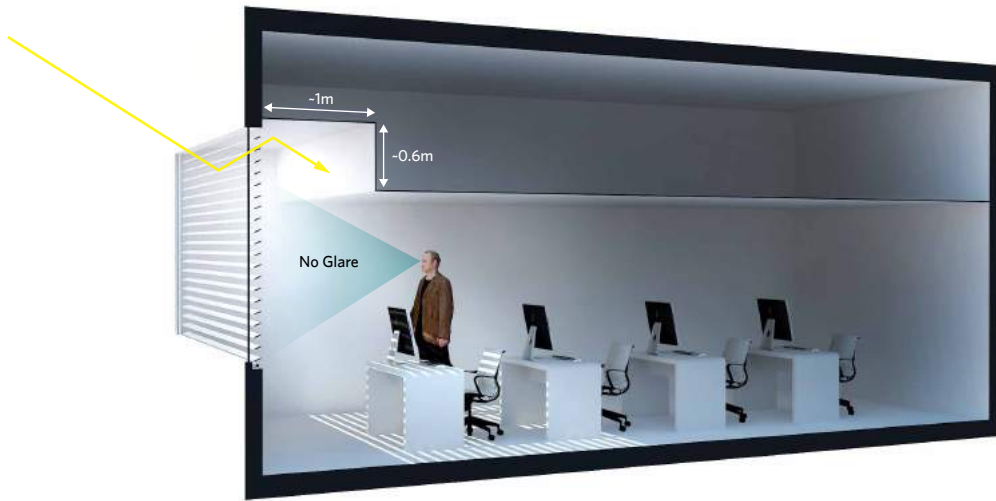
FIGURE 4.5.6 | DAYLIGHT DISTRIBUTION BLOCKED BY DROP OF FALSE CEILING BELOW THE TOP OF WINDOW HEIGHT
