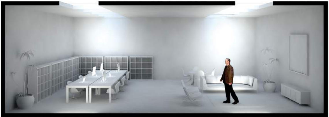
FIGURE 4.6.1 | TYPICAL SKYLIGHT DAYLIGHT HARVESTING
