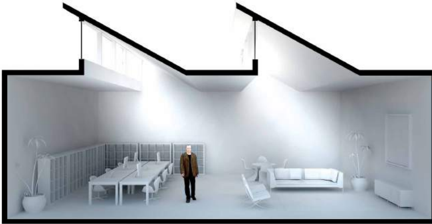
FIGURE 4.6.2 | TYPICAL SAW-TOOTH ROOF LIGHT DAYLIGHT HARVESTING
