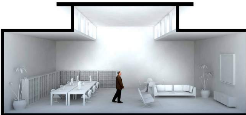
FIGURE 4.6.3 | TYPICAL ROOF MONITOR DAYLIGHT HARVESTING
