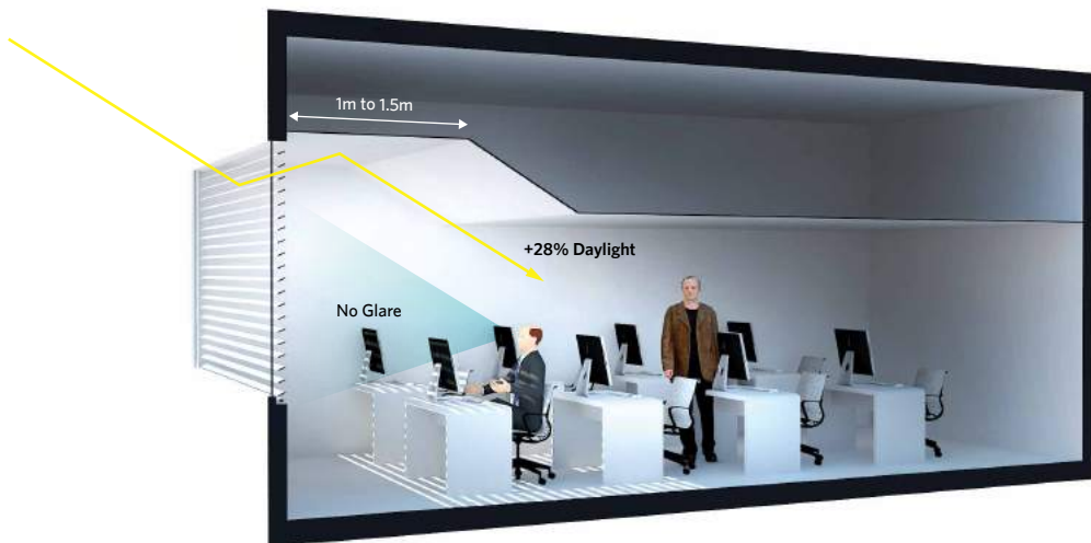
FIGURE 4.5.7 | DAYLIGHT ILLUMINATION LEVEL IS 28% HIGHER THAN FIGURE 4.5.6
